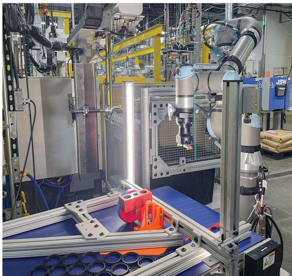
A cobot outfitted with a camera to ensure proper orientation picks up plastic inserts for PUR overmolding. Source: Plastics Technology
