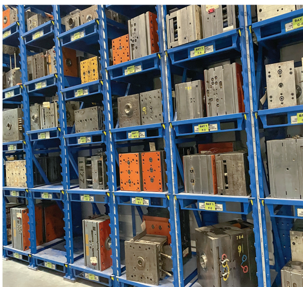
AIM Processing maintains around 700 active tools, recently organizing them via Vidmar tool storage system. Source: AIM Processing
