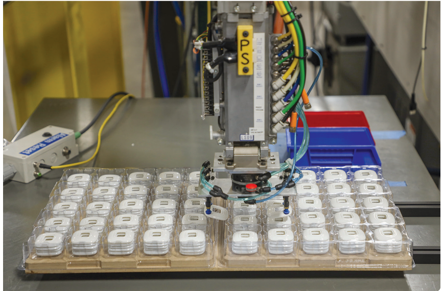
AIM Processing designs and builds its own end-of-arm-tools, according to Gelston, creating an in-house store of components for a "grown-up Erector set." Source: AIM Processing
